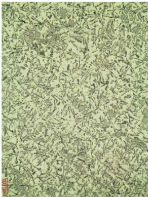
Etial 160 Aluminum Magnification: 100 x
