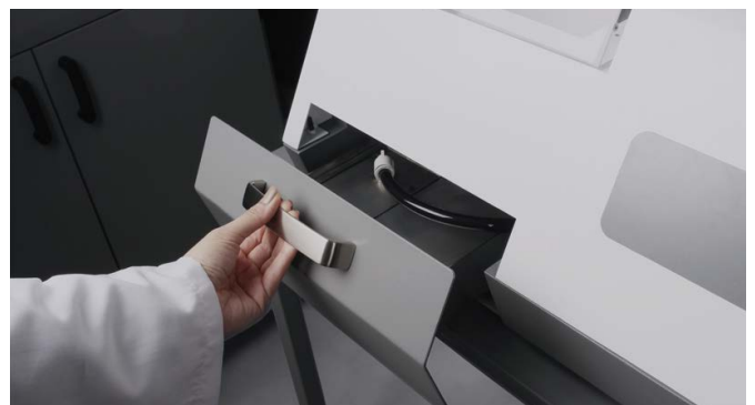
Integrated Cooling Tank
